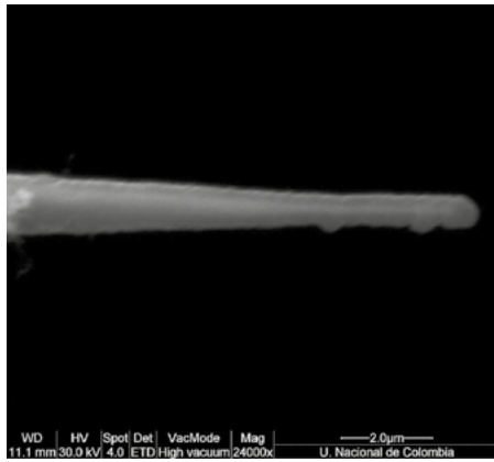
Figure 7. SEM image of the tip-radius obtained with 2mm of immersion.
